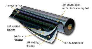
A tough, non-woven, reinforced polyester mat, coated on both sides with Armourplast modified bitumen, to a nominal thickness of 3.8 mm (150 mil). A thin, light, protective thermo-fusible film (which will disappear during heat-welding), is bonded to the underside of the membrane.
